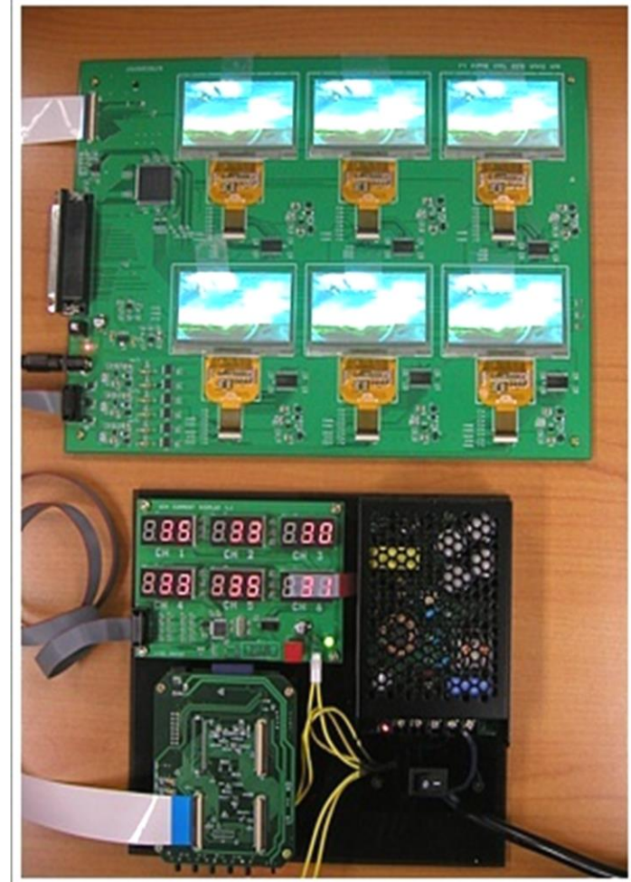
OLED 신뢰성 Board Control System
